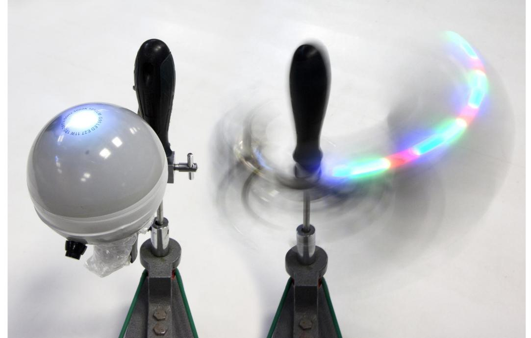
Three LEDs (red, green and blue) light up alternately for 5 ms each. When the assembly is not moving we observe white color, but when it is rotated we observe repeatedly red, green, and blue colors. Why?
