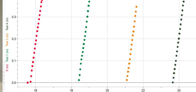
Density of the liquid Measurements were done with well known methods, but also by determine the terminal velocity of a sphere.
