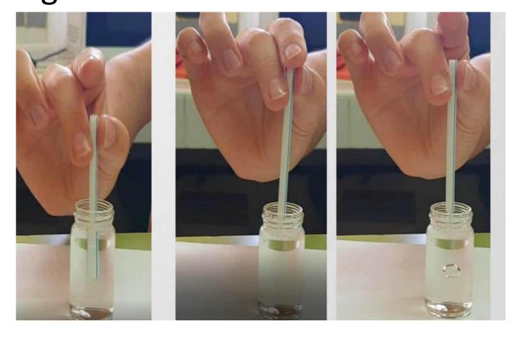
The thickness of the air layer can be calculated geometrically: it is observed that for a real air layer of 1 mm, there is an apparent air thickness of 9 mm
