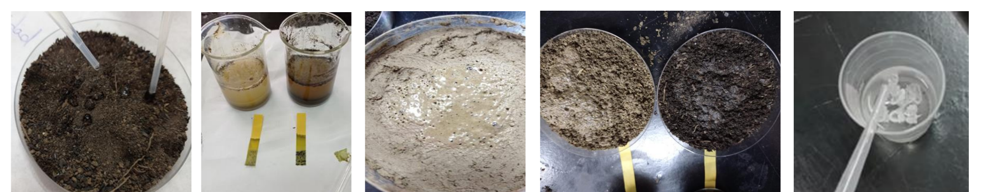
Hydrophobicity, pH comparative, presence of organic matter, presence of carbonates and detection of microbial activity.
